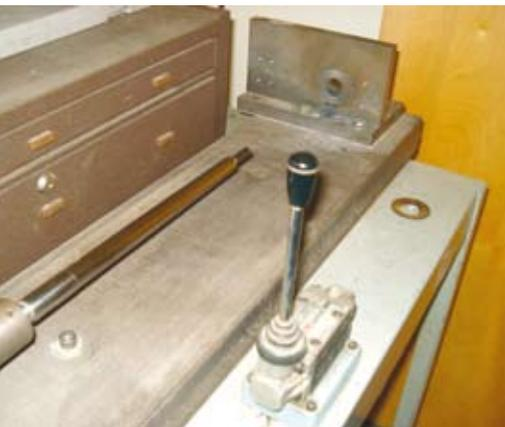
A headjoint mandrel on a hydraulic press, preparing to make a tapered tube. The once-only sheet steel die is visible on the right. The traditional method of forcing a tube onto a mandrel was through a lead ring. Makers today use dies as above, or else dies made of other metals or even plastic.
