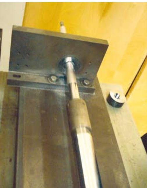
the headjoint tenon to the centre of the embouchure hole, the tube must taper 1.5 to 2mm. Again, through experimentation flutemakers have found that a non-linear—or curved—taper works best. We'll look at this again at the end of the article.
