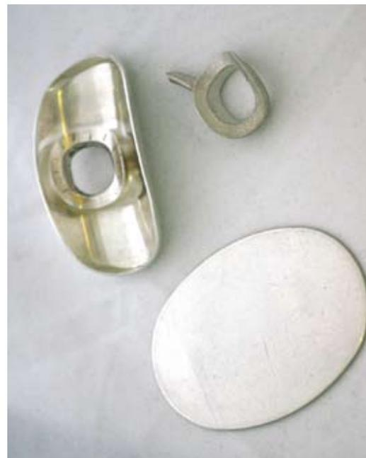
Lip-plate parts: A complete lip-plate, a silver casting for the riser and a silver blank ready to be stamped into a lip-plate.
